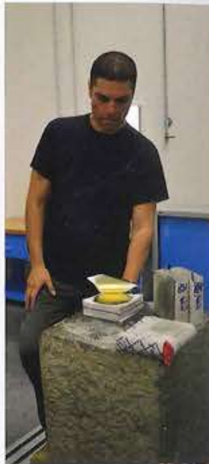
Gold leaf and catches on traditional goldbeating granite block
